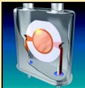
measurements. The sensor consists of a pair of electrodes that support the QCM sensor. When voltage is applied to the sensor, a very stable oscillation occurs.
