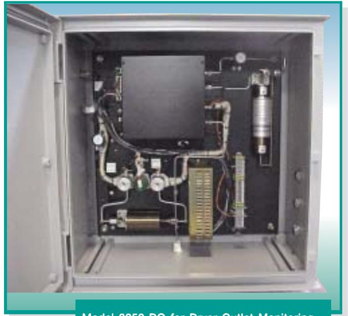
Model 3050-DO for Dryer Outlet Monitoring
